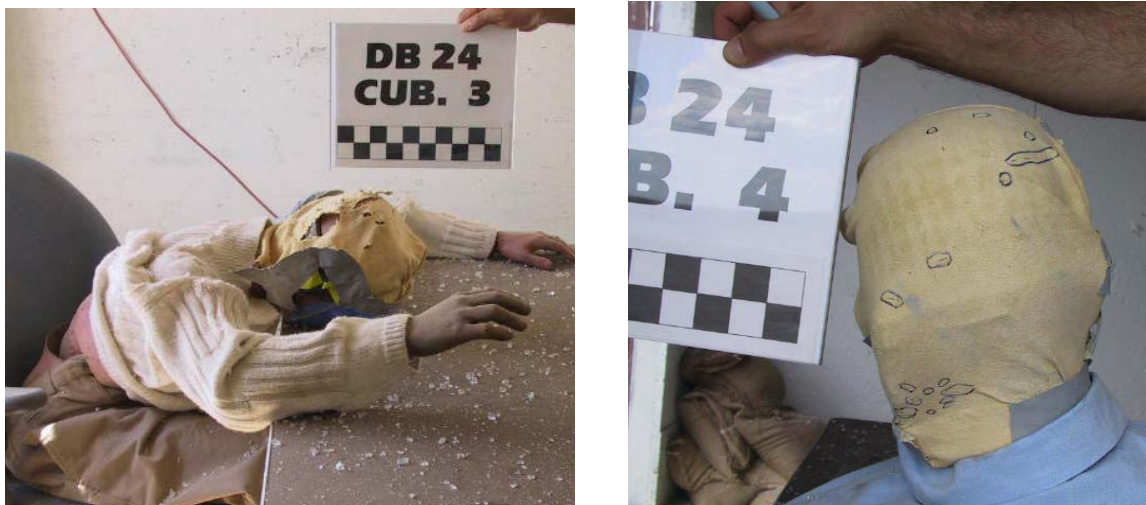
Figure 6. Tears in chamois over ATD heads from unfilmed TTG fragments in DB 24 / 3 and DB 24 / 4.
