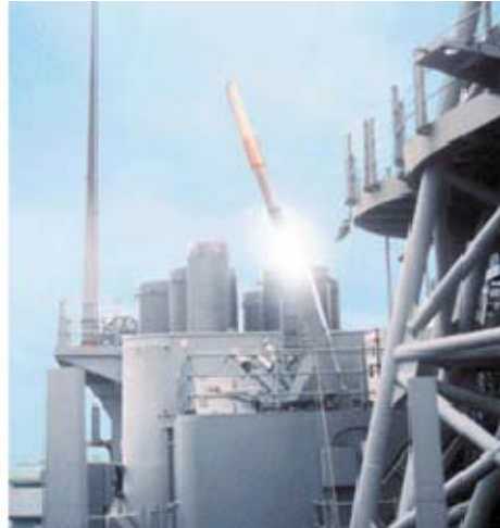
Figure 11. Nulka Launcher Deploying Decoy (From U.S. Navy, n.d.)
