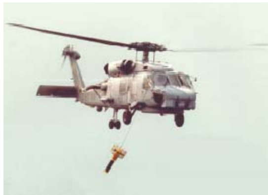
Figure 13. An SH-60B Seahawk Helicopter Fitting with a LAMPS MK III Dipping Sonar (From Pike, 2005d)
