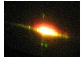
Figure 3: First light from the QPM-based OPO device. Parasitic red and green lights can be observed.
