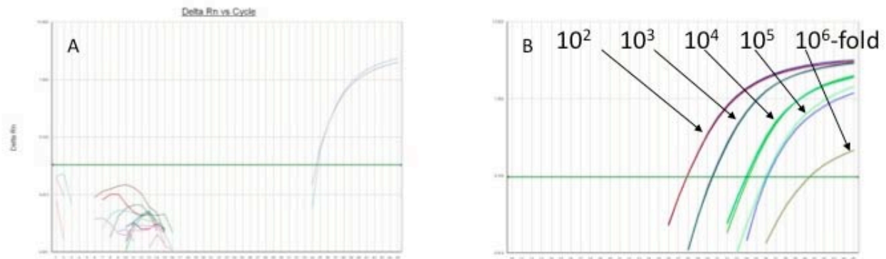
Fig. 10: Developing a sensitive quantitative PCR for detection of XMRV DNA. (A) Amplification of varying amounts of XMRV DNA added to fixed amounts of human placental DNA. Efficient and consistent amplification is seen when at least 50 copies of XMRV genome are present in the reaction. (B) XMRV-infected cells are mixed with uninfected cells at different ratios (1 in 10 2 to 1 in 10 6 ), fixed in formalin, embedded in paraffin, and then sectioned. One such section is mixed with 9 sections of human prostatic tissue, and DNA is prepared from the mixture. XMRV is efficiently detected in the sample that has 1 infected cell in 10 5 , further diluted at least 10 fold in prostate tissue.
