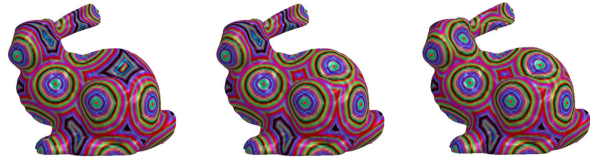
Figure 2: Wave propagation for the incremental computation of discrete intrinsic bounded Voronoi diagrams and thus progressive intrinsic (red) farthest sample point localisation of 21, 23 and 25 sample sites on a triangulated surface (from left to right).
