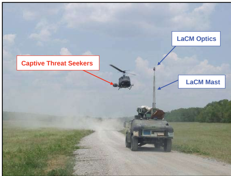
FIGURE 9 LaCM testing with captive seekers on helicopter.
