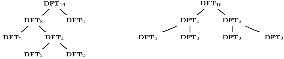
FIGURE 4.2: Two fully expanded ruletrees for \mathbf{DFT}_{16} .
