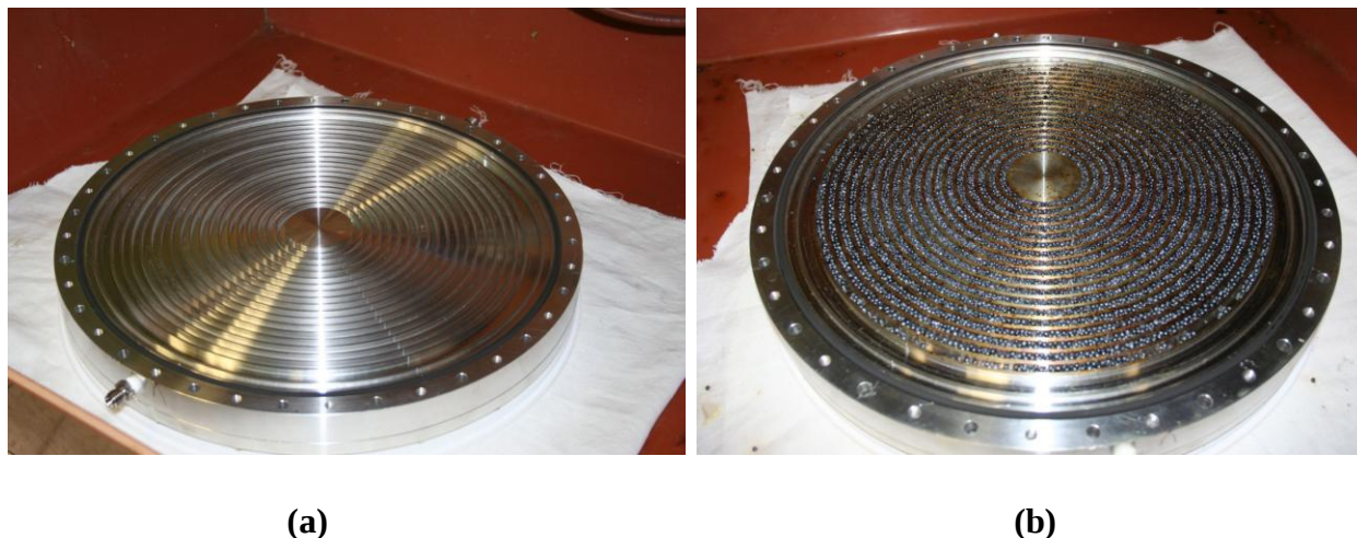
Photo 3. Bottom disk of the I 2 evaporator; without solid I 2 (a) , with I 2 in the grooves (b)
