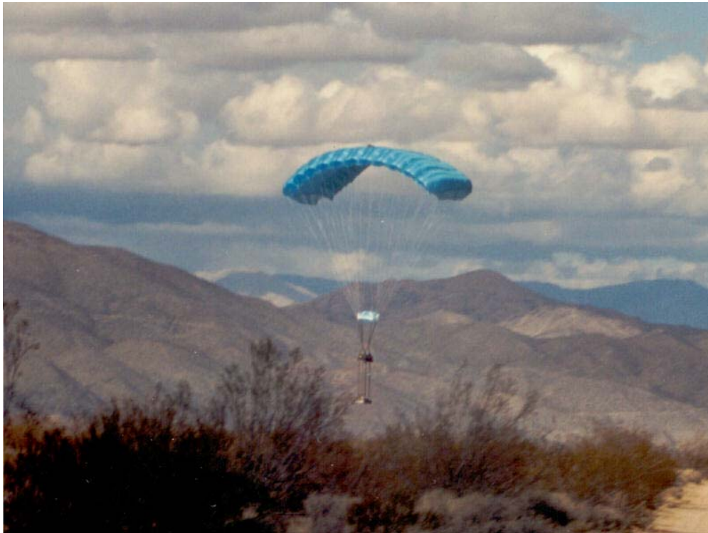
Figure 2 Double-skin 650sq.ft parafoil with 500lb payload
