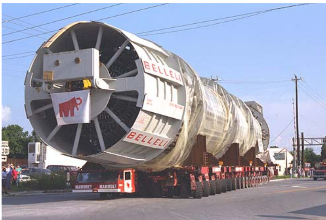
Figure 39. Transporting Tampa Gasifier
