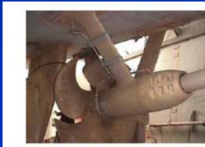
Ship shaft failed after 18 months of service requiring dry docking.
