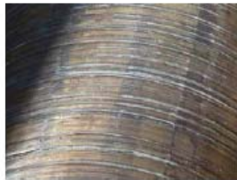
Uncoated shaft experiences severe scoring damage
