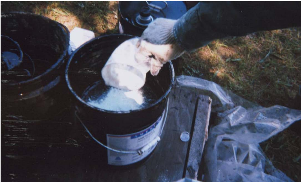
Figure 10. Mixing of fluorescent additives into coal tar epoxy formulation, prior to application.
