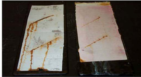
Fig. 6. Samples subjected to ASTM D-5894 Standard Practice for Cyclic Salt Fog/UV Exposure of Painted Metal, (Alternating Exposures in a Fog/Dry Cabinet and a UV Condensation Cabinet) Exposure for 2016 hr. Left: Control coating (with no microcapsules). Right: Self-healing coating with microcapsules containing camphor and red dye
