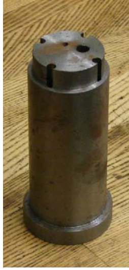
Figure 3. Modified closure cap/steel slug insert for closed bomb volume reduction.
