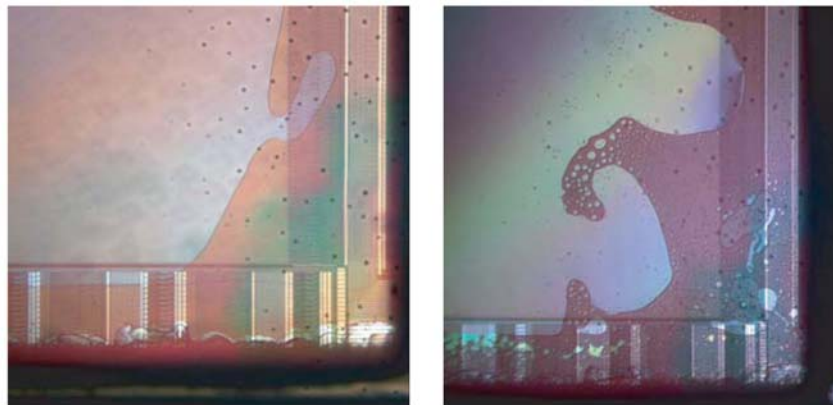
Figure 10: Microscopic images of the lower-right region of a BNS OPA before (left) and after (right) all high-power-CW-laser experiments.
