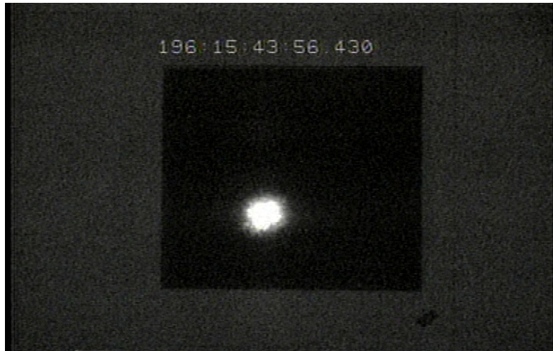
FIGURE C.1-1. Sample Recorded Laser Spot for VBLSS Processing
