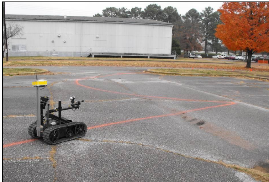
Figure 7. TALON on path following course.
