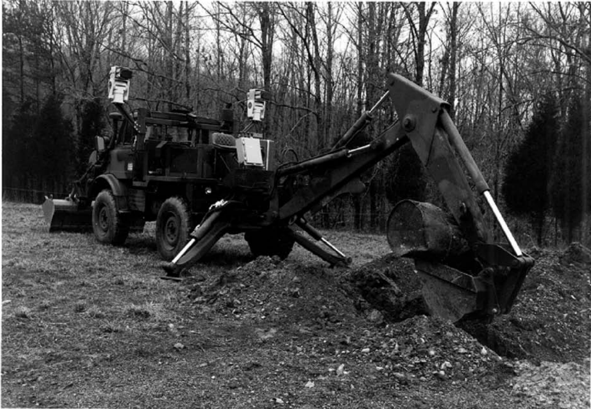
Fig. 1 Telerobotic Small Emplacement Excavator photograph during a backhoe teleoperation demonstration in December 1992 at ORNL. Retrieval of a buried 55-gallon drum was used to simulate buried waste or unexploded ordnance retrieval.
