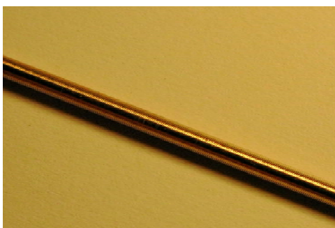
Figure 13. First example of a metawire fabricated using micromachining (pitch 0.4 mm).
