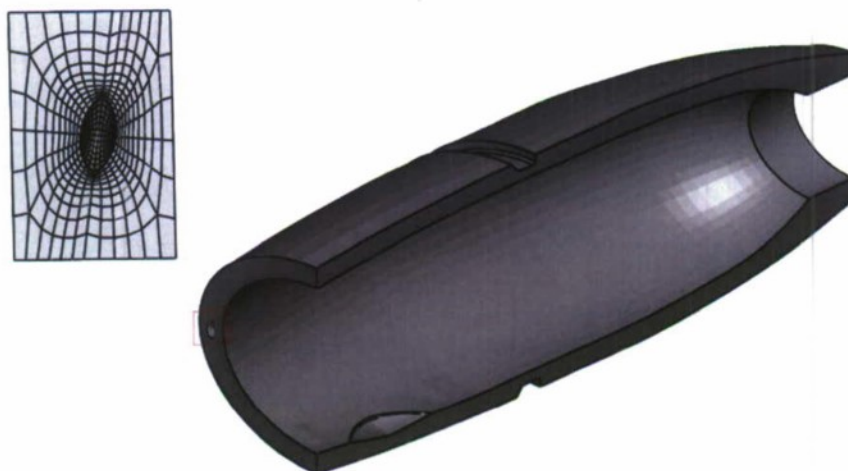
Figure 6 Location and finite element mesh of internal flaw
