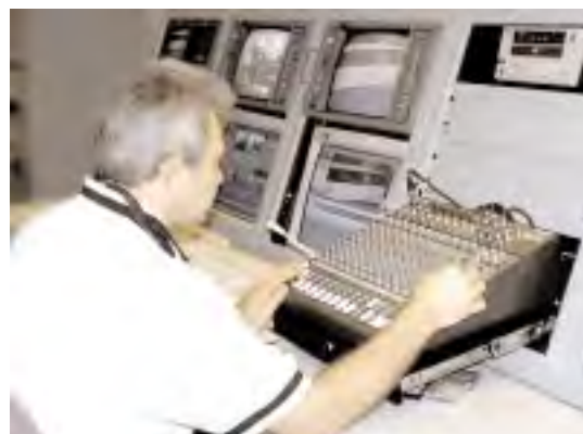
Above: The main rack contains six video sources, a dubbing station, routing hardware, and the base station for one of the nonlinear editors. The studio can accommodate eight different videotape formats and a variety of digital files.
