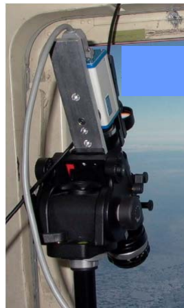
Figure 2. MASCOT [ The image shows the volume scattering function measuring device MASCOT and highlights the 17 independent scattering detectors (sd) and lasor source (ls)]
