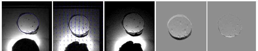
Fig. 1: Representative registration results for prostate phantom images. (a) reference image (b) source image overlapped with the displacement obtained. (c) registered image. (d) difference between the segmented reference and source. (e) difference between the segmented reference and the registered image.
