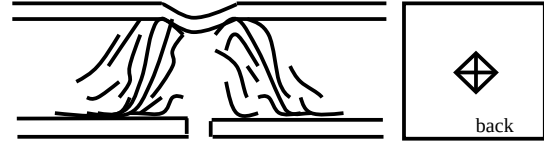
(b) Back facesheet failure.
