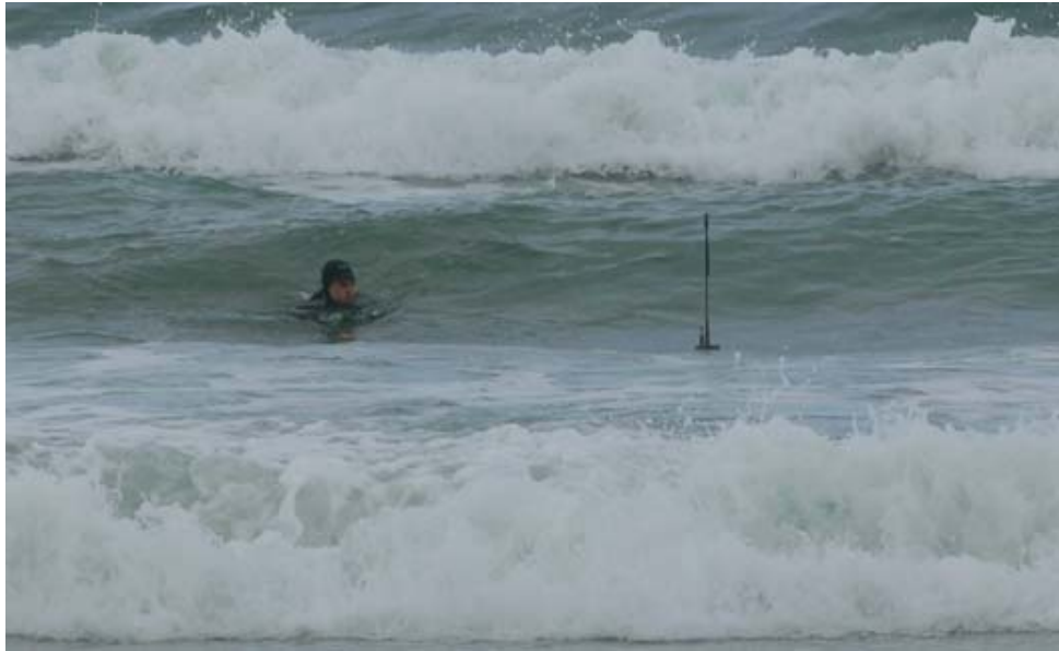
Figure 3: GPS equipped, water-following drifter in the surf zone. The drifters, that 'duck under' bores and do not surf shoreward, relay their position to shore, allowing real-time tracking.
