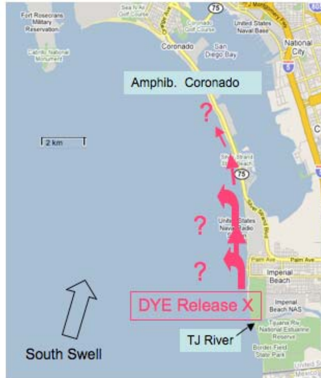
Figure 6: Schematic of the IB09 plume experiment with South swell. Dye injected continuously near the shoreline is advected north by the breaking-wave driven alongshore current. A fixed array of instruments at Imperial Beach spans from the shoreline to about 5m depth. The jetski sampling pattern is similar to figure 3 (right) but expanded to cover several km of dye plume. A small boat is sampling offshore.
