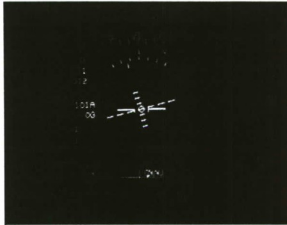
Figure 1: Head up display symbology superimposed on night vision goggles (ANVIS).
