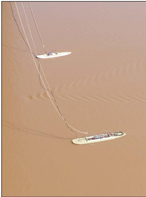
Figure 2: Photo of the instrumented surfboards deployed from the bridge in the Petitcodiac River. Upper board consists of a 1.2 MHz RDI ADCP and a Dual Frequency (50 and 200 kHz) Knudsen sounder. The lower board has a 2.5 MHz rotary sonar and 1.2 MHz RDI ADCP mounted on it. The wake between the boards is caused by a SUBS package just below the surface.
