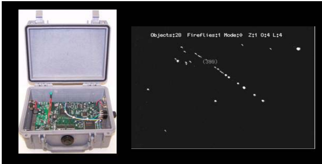
Fig. 1: Prototype electronics used to process video signals to locate and decode optical signals, and a representative screen capture showing the detection of a signal source placed near many noise sources.
