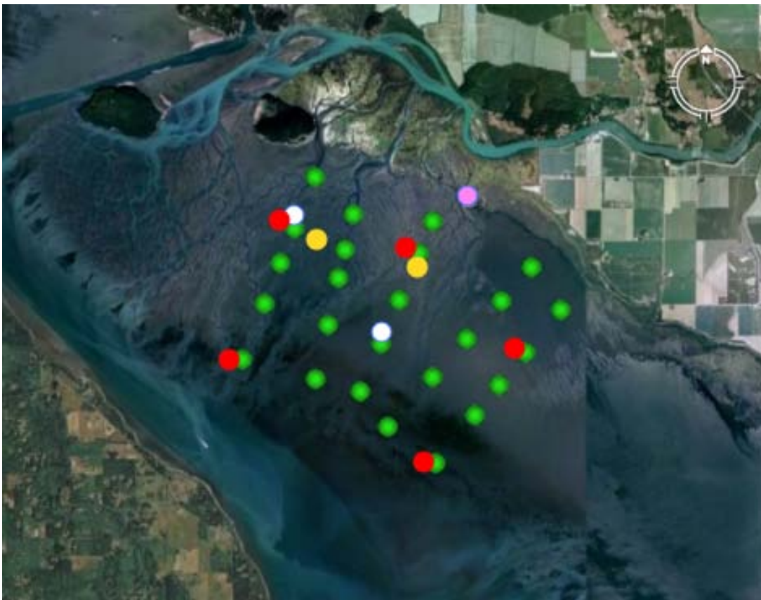
Figure 1: Approximately 5 by 5 km array of 25 bottom-mounted tripods (green symbols, each with an acoustic current meter, pressure gage, and CT sensor), 2 meteorological stations (white), 5 colocated current profilers and floating CTD stacks with sensors about 20 and 70 cm below the water surface (red), and 2 colocated current meters and pressure gages (yellow) deployed in 2009. A meteorological station also was deployed on Craft Is. by J. Thomson (UW-APL) (pink).
