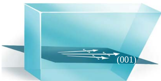
Fig. 5.1.3. Polarization of the divergent slow shear wave beam propagating in plane (001) of \text{TeO}_2 .
