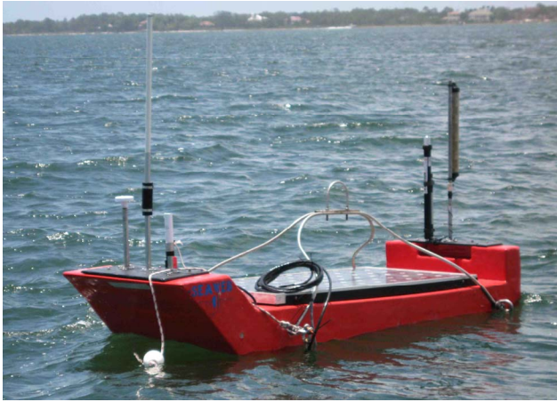
Figure 4. A moored Seaweb Racom gateway buoy.
