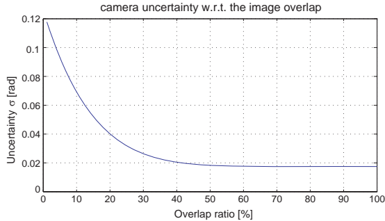
(b) Standard deviation of the camera measurement noise as a function of the overlap ratio
