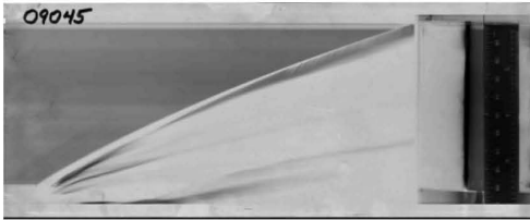
Figure 3. The streak image shows the propagation of a shock into PMMA. Time increases from the left to right and the propagation from bottom to top. The shock front is tracked for experimental and numerical comparison.
