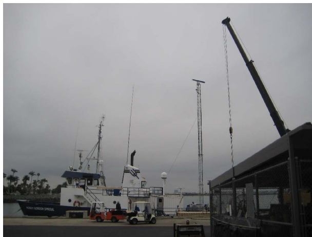
Figure 5. Photograph of the R/V Sproul dockside with the X-band radar tower installed. The tower is designed to be above all other objects so that it has a clear field of view.
