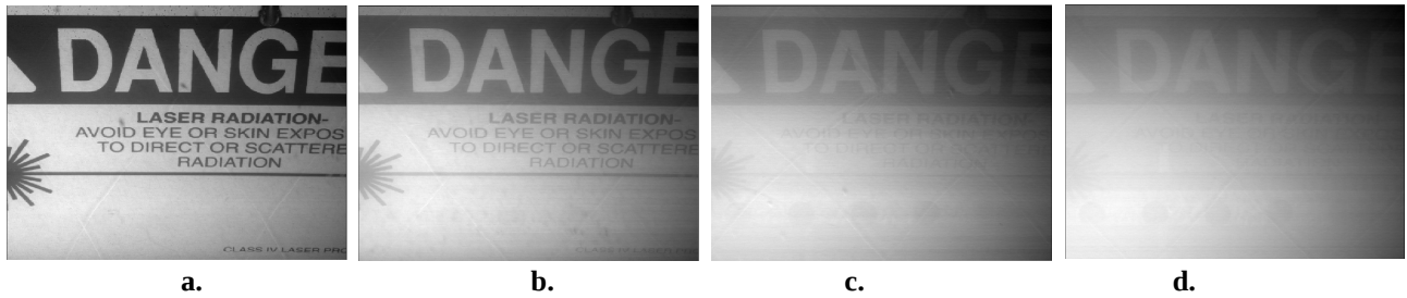
Fig. 7. Images generated with the DC component of the signal detected by the PMT for different water turbidities: 7a - cR=5.2 , cr=1.1 ; 7b - cR=13 , cr=2.7 ; 7c - cR=21 , cr=4.3 ; and 7d - cR=24 , cr=4.9 .
