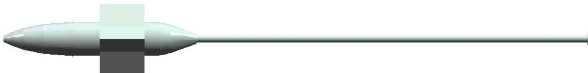
Fig. 1 Schematic view of a STING penetrometer with a single extension rod and a small foot
