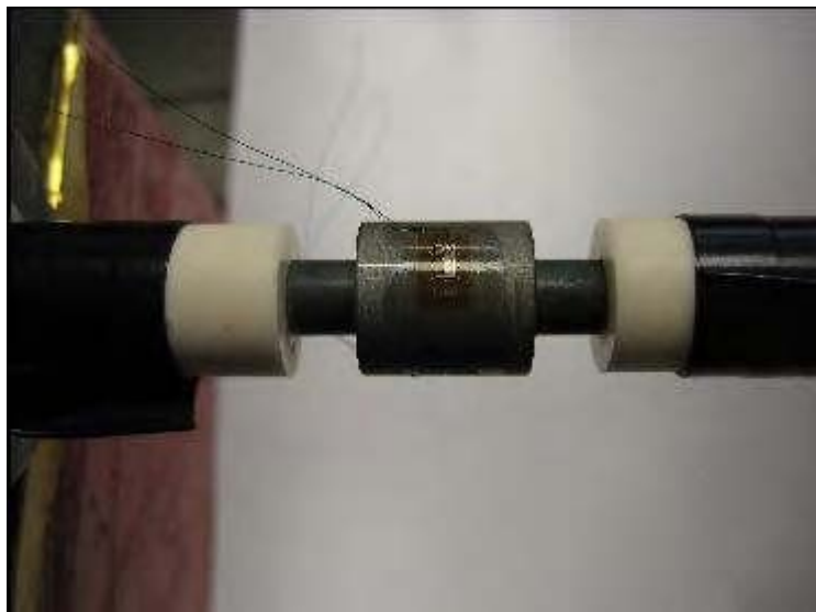
Figure 3. Confined sleeve test placed in the split-Hopkinson bar.
