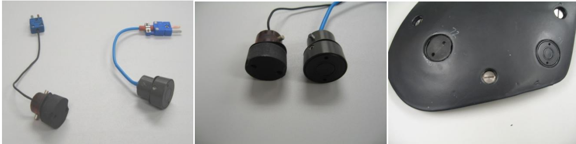
Figure 6: Recommended ceramic (l in each photo) or copper skin-simulant sensors (r in each photo).
