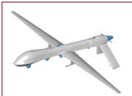
Figure 2 A FASTGEN Model was Developed for the MQ-1
