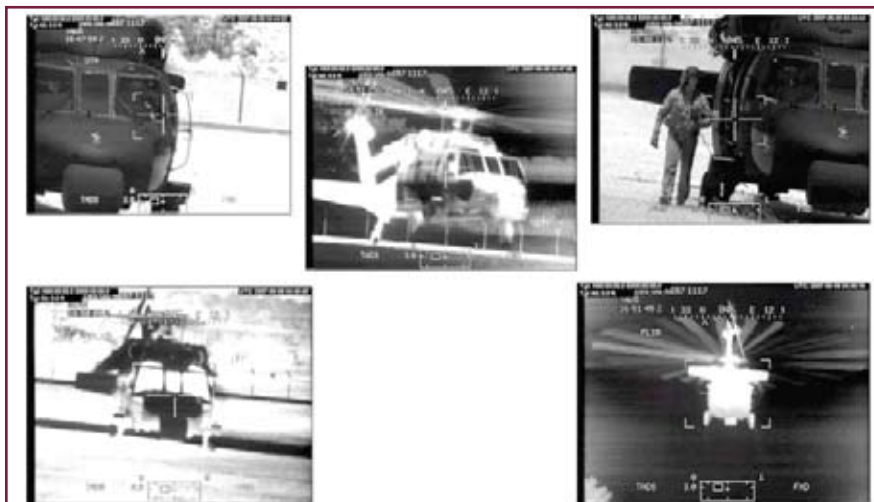
Figure 8 AH-64D TADS Video as Viewed and Recorded on Ground OSRVT Toughbook Computer After Transmitted Via MTCDL System From AH-64D Aircraft to Ground OSRVT Station
