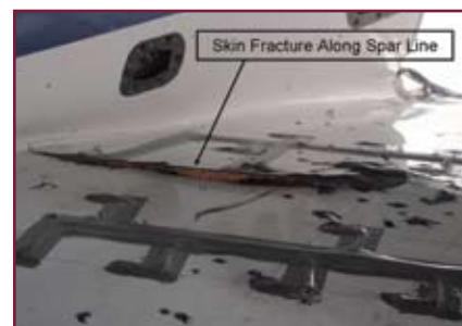
Figure 3 HEI Dry Bay Damage
