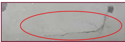
Figure 7 Damage to UAS Fuselage Section
