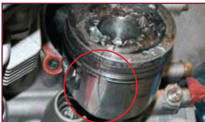
Figure 6 Crack in Side of Piston
