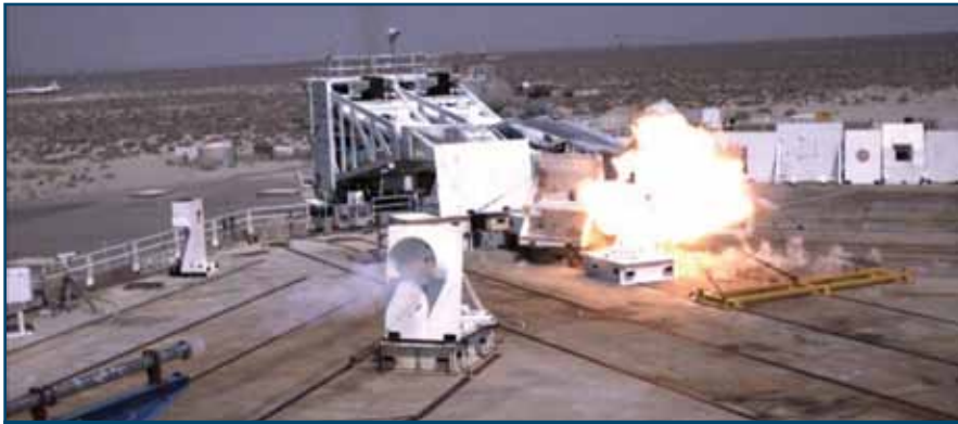
An F-18 is hidden behind this explosion during the first live MANPADS launch using an operating aircraft with realistic intercept velocity, and realistic airflow provided by the Weapons Survivability Lab's High-Velocity Airflow System at NAWCWD China Lake.
