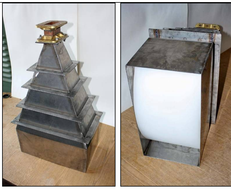
Fig. 3.17. Newest irradiating horn with two polythene lenses inside
