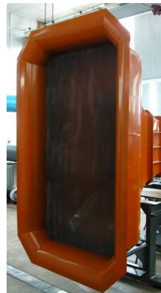
Fig. 2.7. Entrance of a nozzle collector with the installed grid
