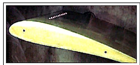
Fig. 2.1,a. The blade- (airfoil-) type model with embedded MW-initiators generating a spanwise-regular array of localized plasma discharges for experimental flow-control investigations in the wind-tunnel facility of Fig. 2.1.
