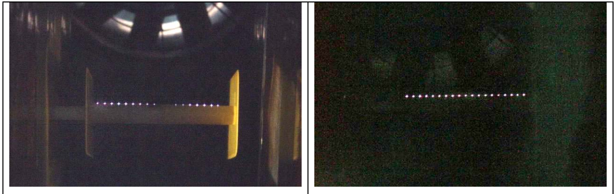
Fig. 3.21. Multiple MWdischarges in the vicinity of the airfoil model surface in wind-tunnel experiments: initial tests (left), and after the system adjustment (right)
