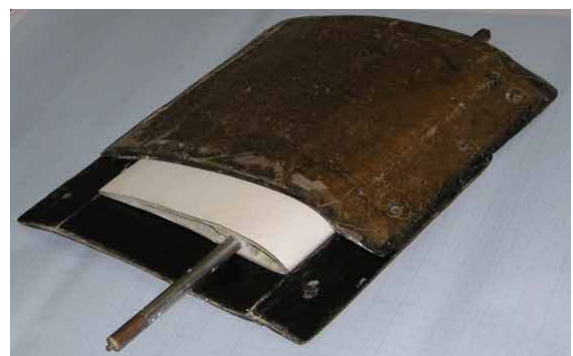
Fig. 3.5. Fabrication of a model body according to the given geometry: the model with a holder within two moulds shaping convex and concave panels of the model.
