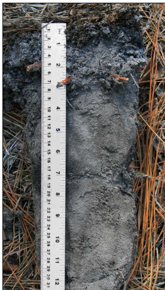
Figure 17. Stripped areas form a diffuse, splotchy pattern in this hydric sandy soil .
