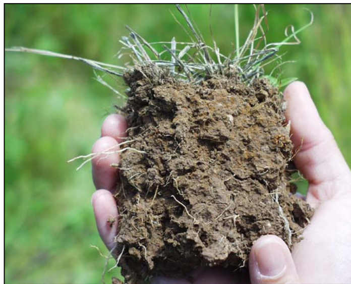
Figure 23. In this example, the layer containing more than 5 percent redox concentrations begins at the soil surface and is slightly more than 2 in. (5 cm) thick.
