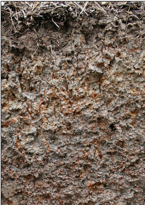
Figure 19. Example of indicator F3 (Depleted Matrix), in which redox concentrations extend nearly to the surface.
