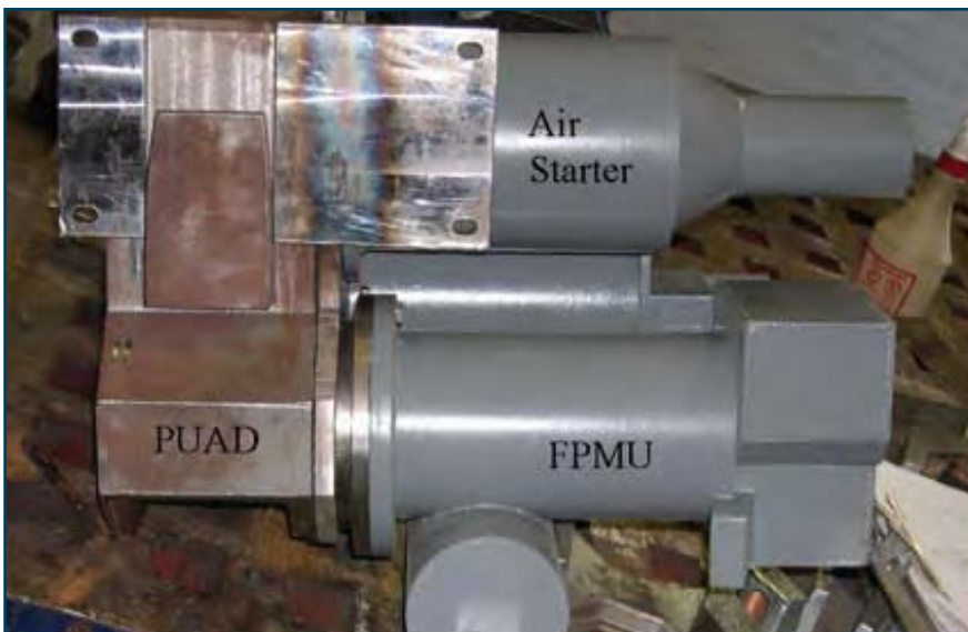
Figure 4 Top View of Replica FPMU and Air Starter Connected to Replica PUAD
