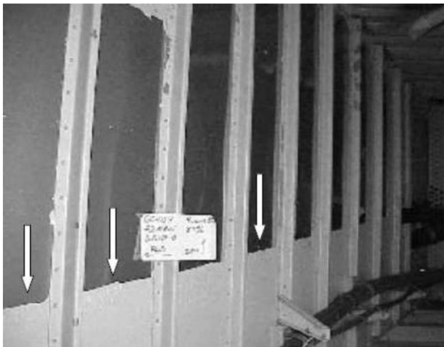
Figure 2. Fuel tank topcoat peeling (FTTP) occurring in B-52 wing tank test panels (Aliband et al., 2006)
