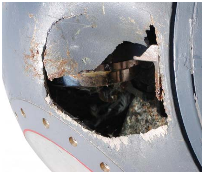
Aircraft damage from bird strike.
