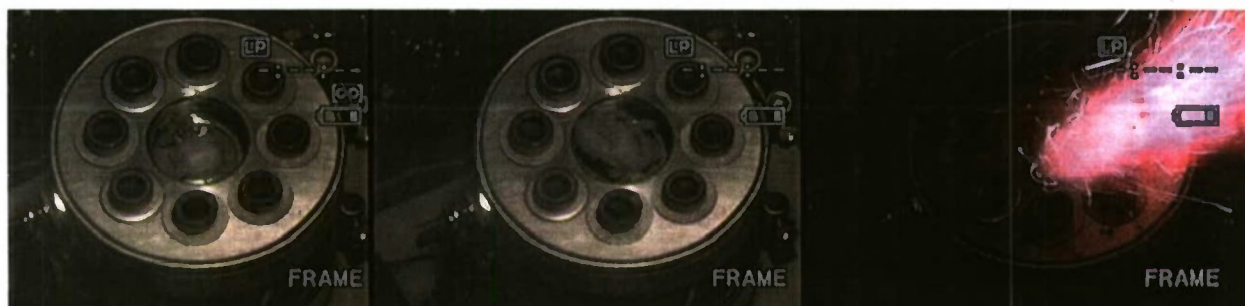
Figure 12 PBXN-109 w/HDPE liner extruding then burning
