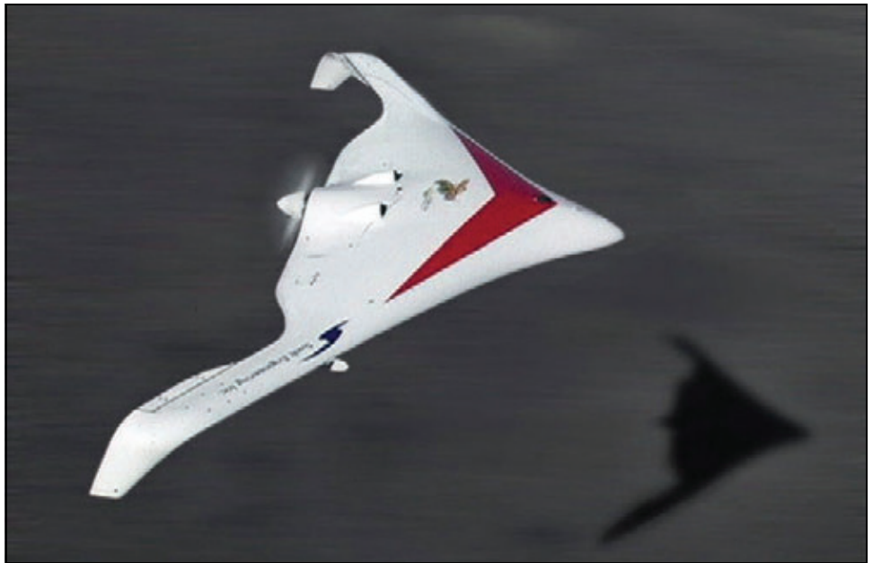
The Swift Engineering KillerBee UAS allows a payload between 14 and 30 kg and can stay airborne for up to 15 hours a useful vehicle for CW detection.
