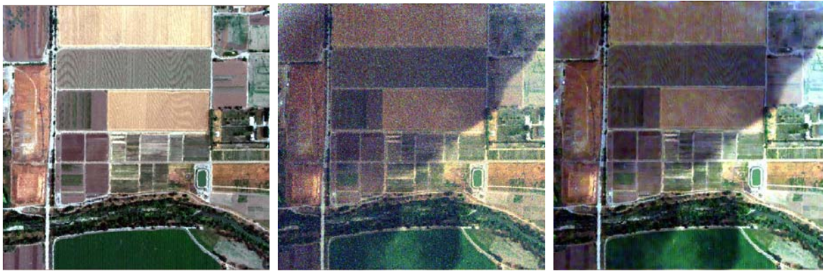
Fig. 8. Davis, CA hyperspectral scene simulations. At left, input surface reflectance; at center, MCSce apparent reflectance output; at right, the result after noise removal.
