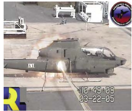
Figure 5. RPG “plasma jet” exiting out the helicopter
