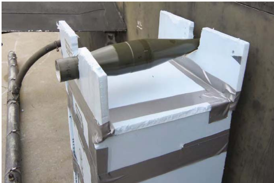
Figure 4. RPG warhead setup for fuel ullage test
