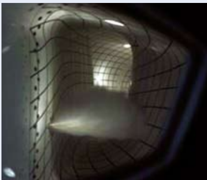
LF-12c fuel ingestion testing of F-135 Engine.
