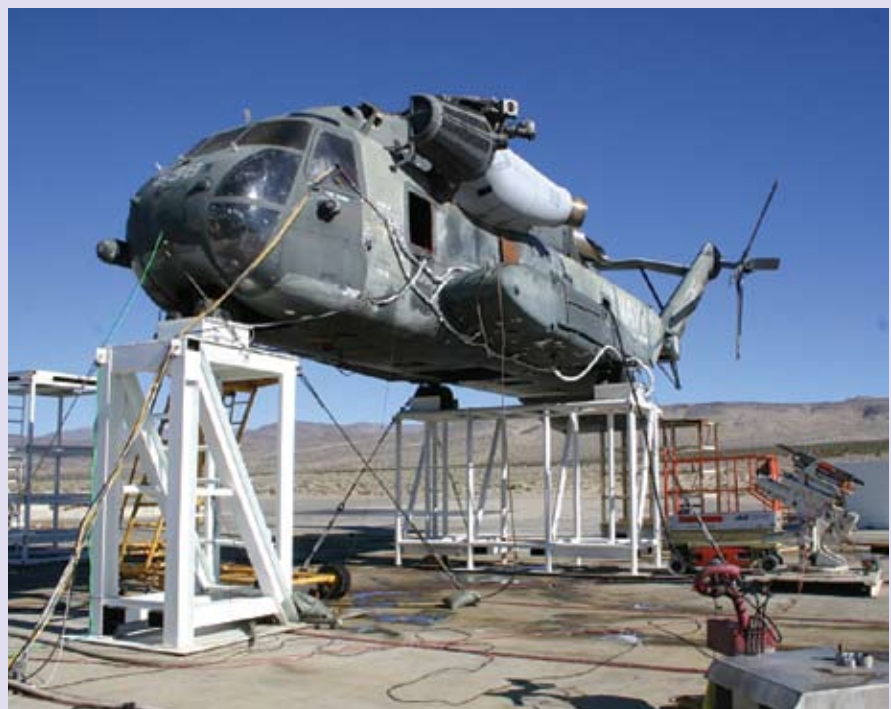
Figure 2. CH-53E fuel systems vulnerability testing (2005).
