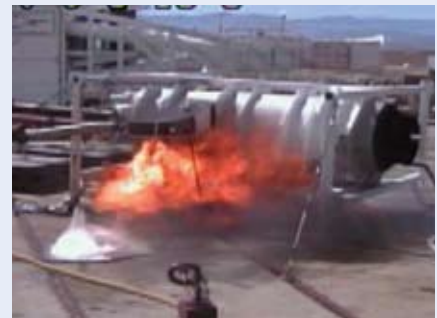
LF-11c roll post bay fire testing.
