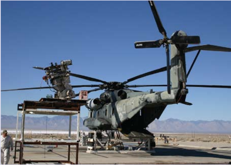
Figure 3. CH-53E tail rotor system vulnerability testing (2006).
