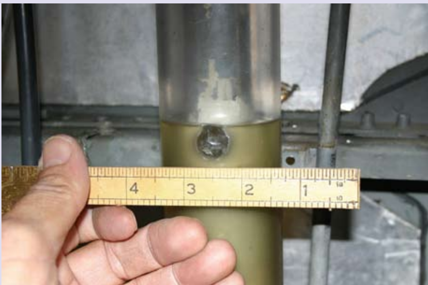
Figure 4. Self-healing plastic fuel line sleeve.
