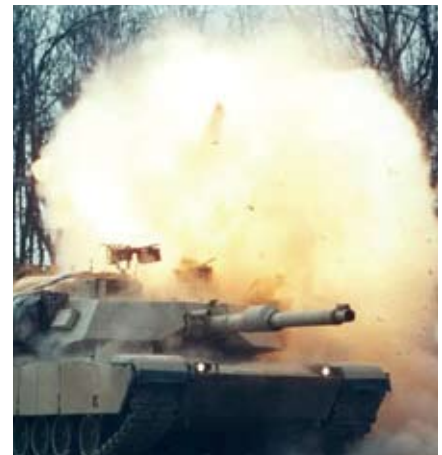
Figure 2. An Abrams live fire test. Realistic testing provides a basis for understanding the effects of combat hits.
