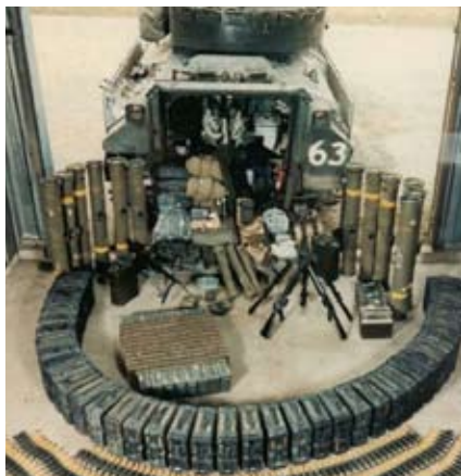
Figure 1. The Bradley was tested in a full-up configuration, with a standard load of fuel and munitions.
