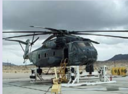
Figure 1. CH-53E rotor and drive shaft systems vulnerability testing (2004).
