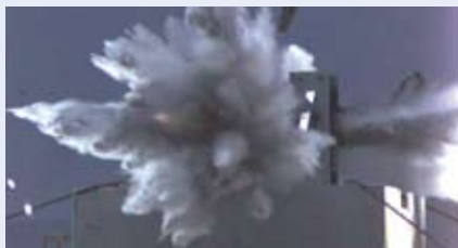
LF-03 HRAM mitigation testing using an F-16.
