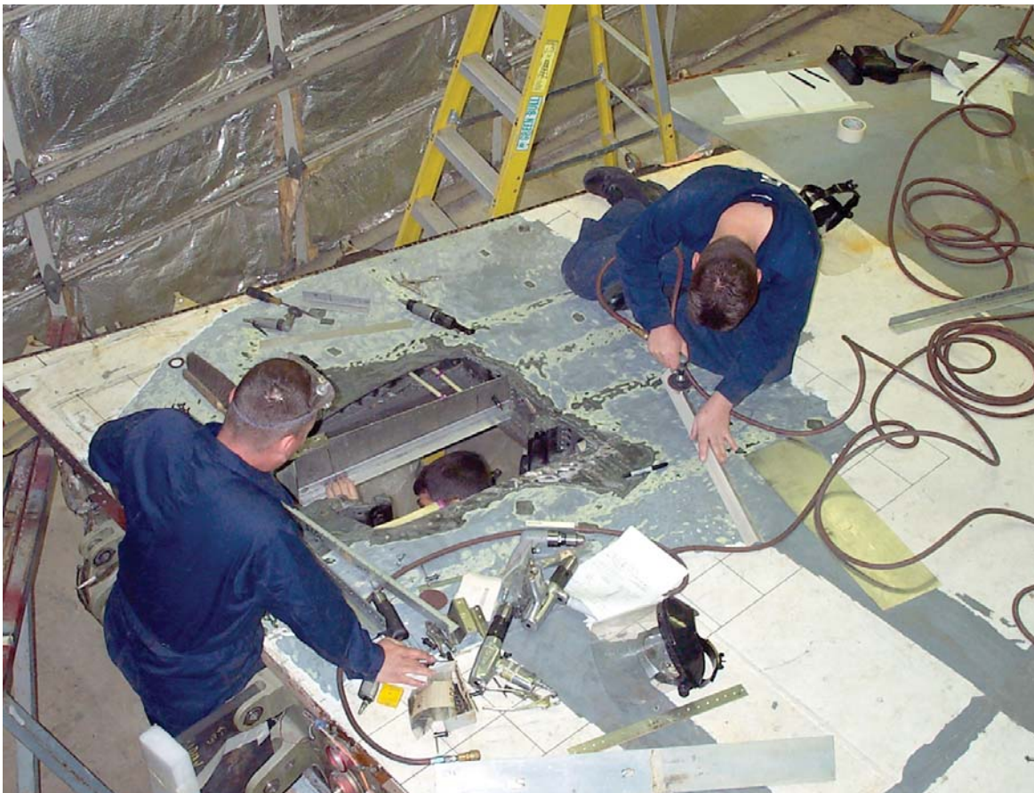
TSgt Tim Fugere (649th CLSS), TSgt Richard Cousineau, and SSgt Sean Dolney (653rd CLSS) manufacture parts to repair the F/A-22 wing structure.
